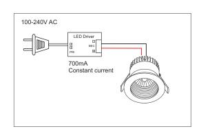
Always disconnect the mains of the LED driver before plugging or unplugging the LED's!! The LED's will be damaged or destroyed because of the high voltage present on the driver output when there is no load connected. Connect the main after all Led's and plugs are connected!
