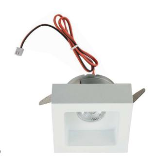
Always disconnect the mains of the LED driver before plugging or unplugging the LED's!! The LED's will be damaged or destroyed because of the high voltage present on the driver output when there is no load connected. Connect the main after all Led's and plugs are connected!
