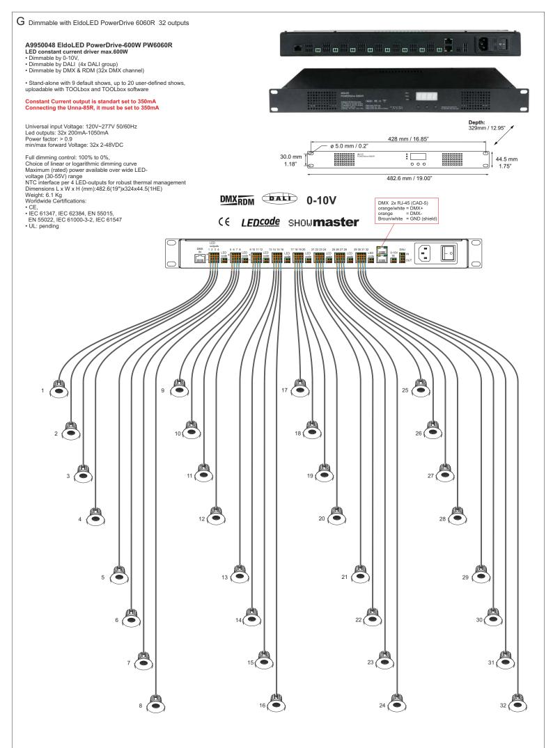
Each connector has 4 outputchannels. Load max. 1x Unna-85R WW to one output-channel and total max. 32 Unna-85R WW to one driver. To avoid damages to the LED, all cables & plugs must be connected before switching on the power !
