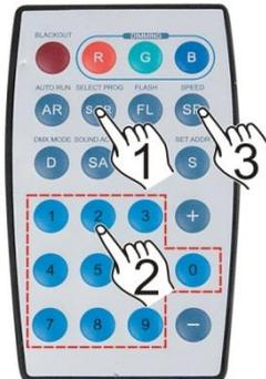
**SP** button (8): Press the speed button to activate the Running Speed function. This function is only available in color jump or color dream Mode. Use the + (13) and - (14) buttons to change the running speed. + = **faster**, - = **slower**
